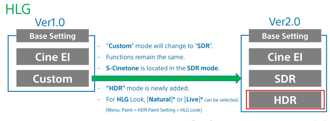
\*[Natural]: Industry standard HLG based on ITU-R BT.2100 (HLG). [Live]: Similar with Sony's system camera HLG.
