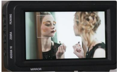
Focus Touch Control allows you to precisely set the camera's specific focus area by simply touching the LCD viewfinder.
